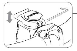
If the SNAP LOCK of your OX is too loose / tight, you can fine-tune it by adjusting the height of the locking hook. Use hex key (2.5mm)
